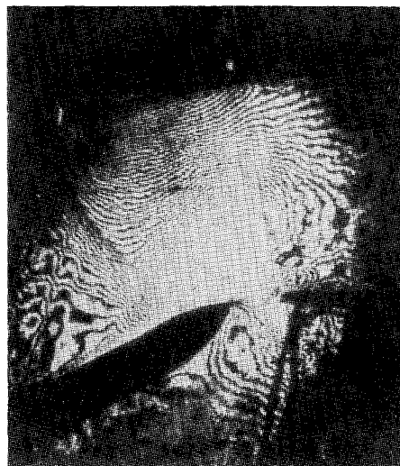
Fig. 9 Interferogram of diffuser entry flowfield.
